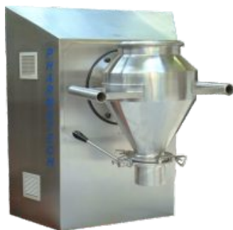
Special AgiBlend AB400 with 75 litre Double Cone
